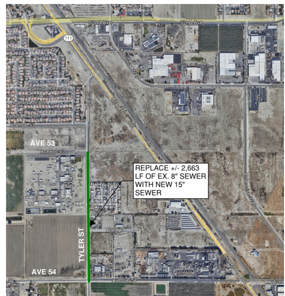
Figure 1: Sewer Replacement Location
